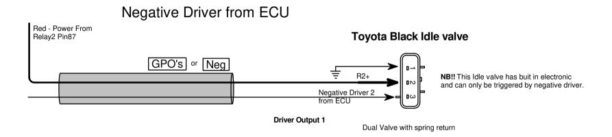
**Note:** The connection to the ECU changes with the GP Output Priority selection. View the Priority spreadsheet for the specific firmware to see which output is selected. It must be a negative driver as the idle electronics has a buit in pull-up resistor.
